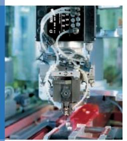
Our new generation of robots. The specialty of this assembly component is the random parts feed, whose positioning is ascertained by the integrated Bosch image processing system.
