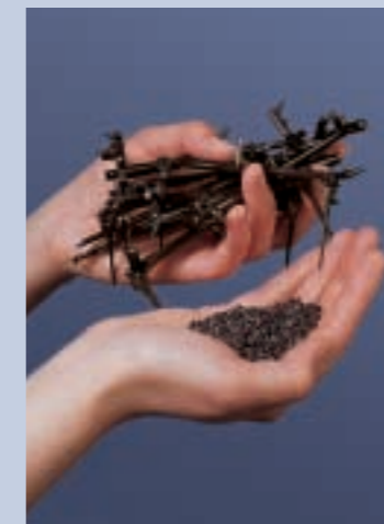
Sprue waste recycling at the Waiblingen plant
