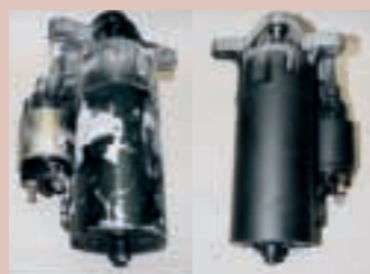
Starter before (left) and after factory reconditioning (right)
