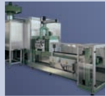
Painting station for hydraulic valve housings
