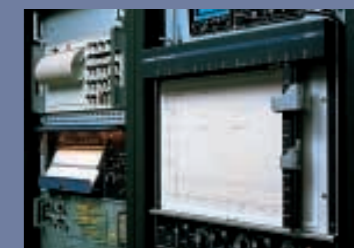
Two measuring devices in the cold cell with XY and UV recorder
