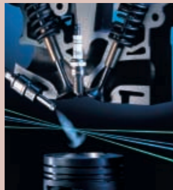
Bosch develops gasoline direct injection systems for almost all European car makers – to further reduce fuel consumption
