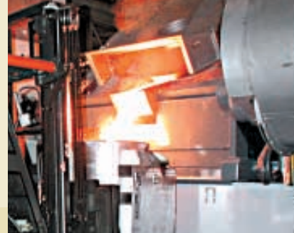
Smelting iron in the new medium frequency furnaces at Bosch Rexroth ▣
